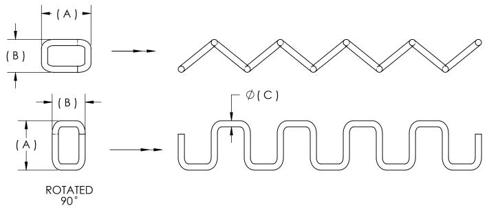
NOTE: THIS SYSTEM MAY BE INSTALLED TWO WAYS TO ACCOMODATE VARIOUS LINING THICKNESSES (AS SHOWN IN END VIEW SECTIONS)
